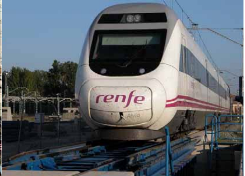
Class 130 Talgo train (left) and class 120 CAF train (right) starting the automatic track gauge changeover
