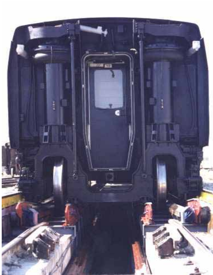
Automatic track gauge changeover without changing axles or bogies
