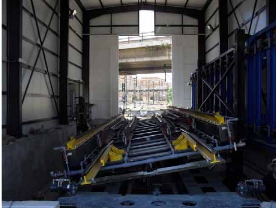
Valencia automatic track gauge changeover for trains (Foto: Sergio López Lara)
