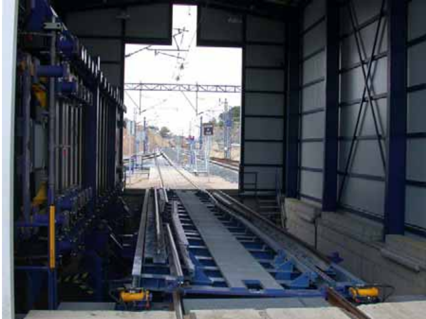
In the third generation changers, the catenary passes through the changer
