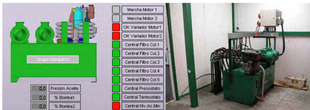
Control system (left) and hydraulic generating set (right)
