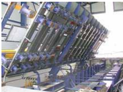
Platform of the Talgo (left) and CAF (right) changers. On the left, a vertically folding platform. On the right, huts for the portable third generation changers
