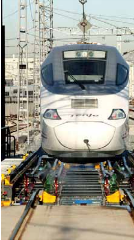
Class 130 Talgo train (left) and class 120 CAF train (right) starting the automatic track gauge changeover
