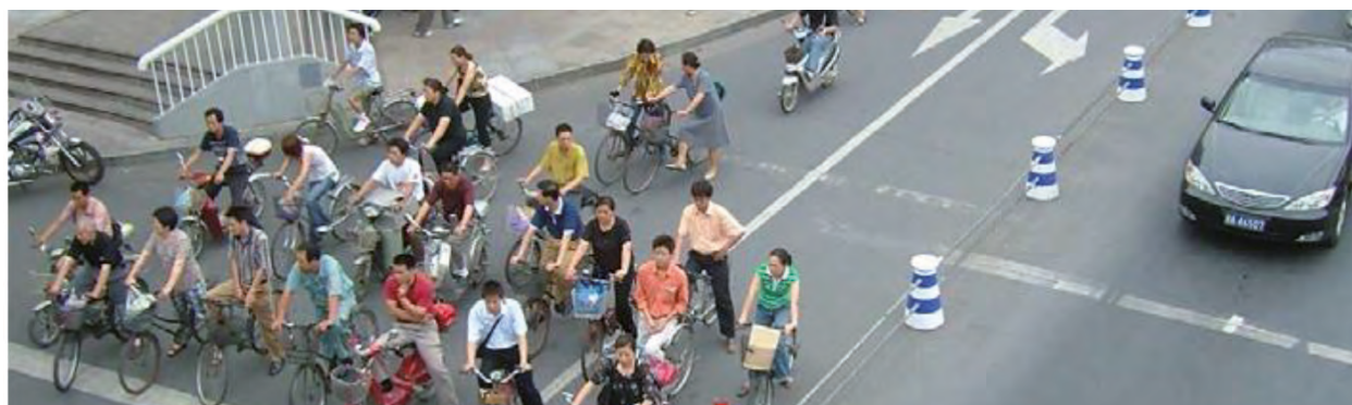
Figure 12: A high capacity cycleway with physical protection, turning lanes and an advanced stop line for cyclists in Hangzhou, China. Source: TOD standard 2.1.
