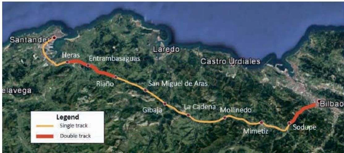
Figure 9. Final layout of the proposed line showing the single- and double-track segments. Santander-Bilbao Case
