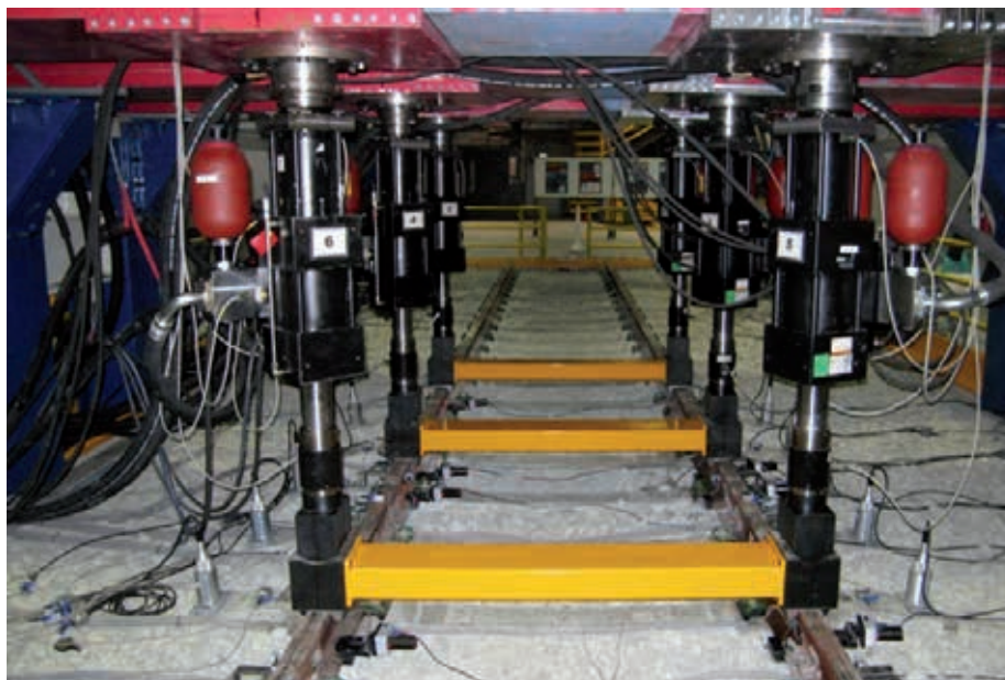
Figure 2. Detail of the hydraulic actuators
