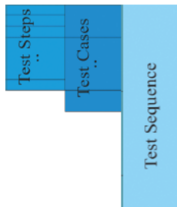
Figure 3: Symbolic structure of a test sequence for conformity testing
