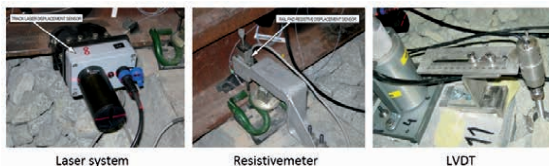
Figure 12. Instrumentation used in the static tests
