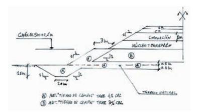
Modified of the soils characteristics in the case of using lime:
