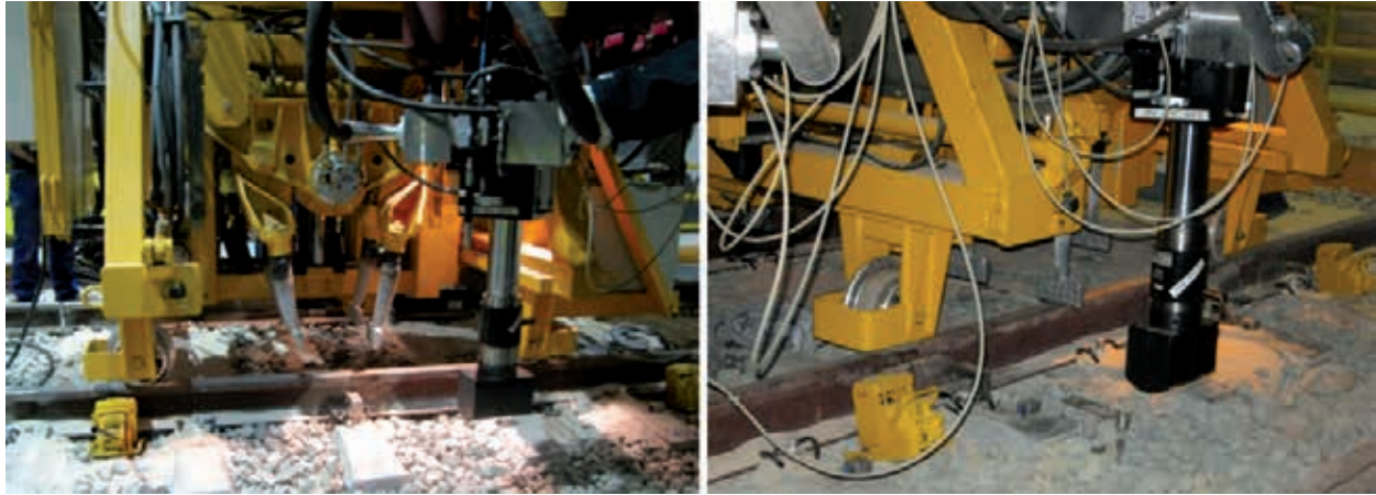
Figure 4. General view of the tamping machine used in CTB
