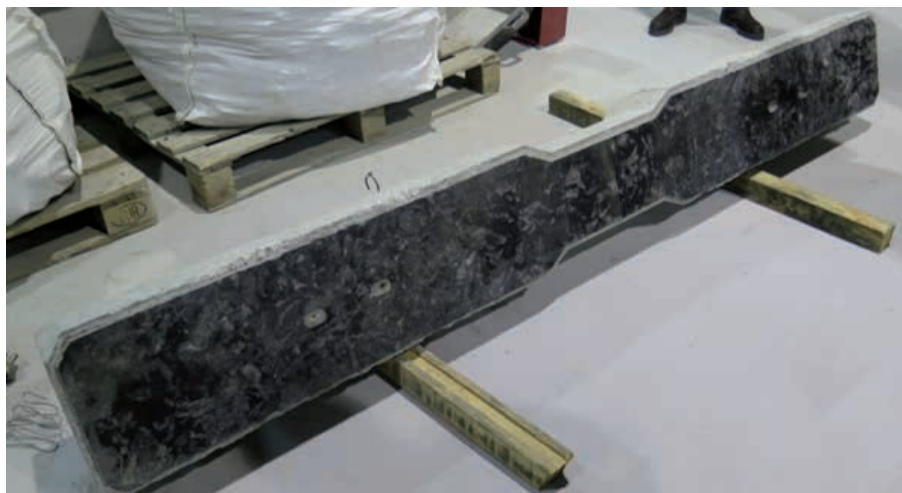
Figure 26. General aspect of USP installed in the sleepers
