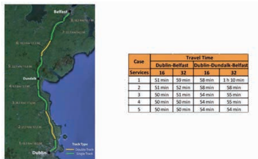
Figure 17. Optimal ADST railway line solution and Travel time comparison of the 5 alternatives considered.)
