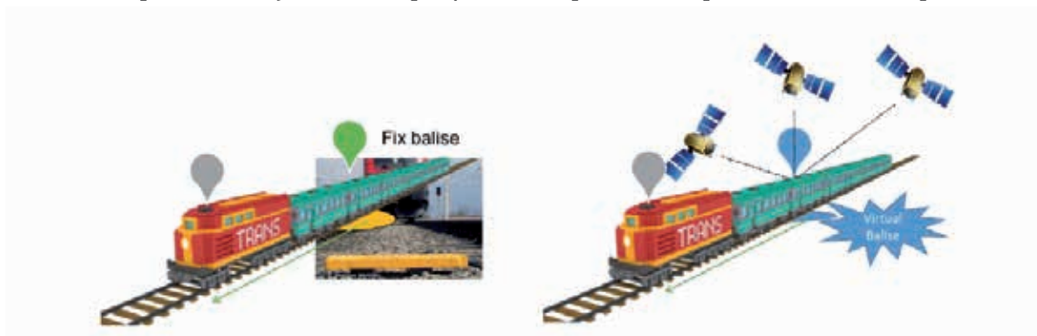
Figure 2. Virtual Balise use instead of physical trackside Balise
